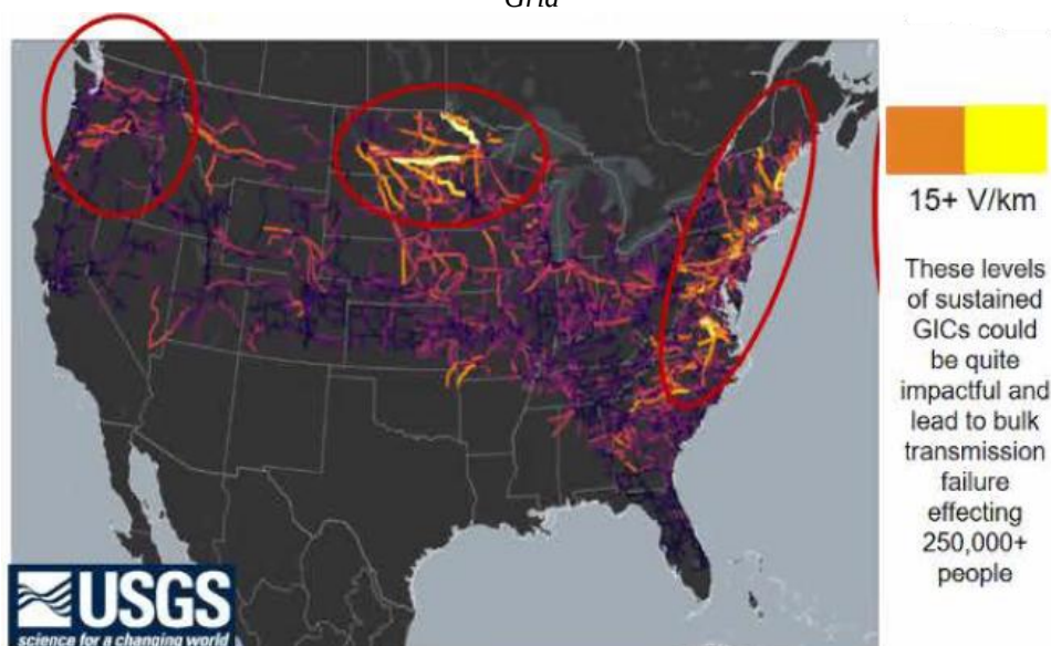
Figure 4.27 USGS Map from the report showing 100-year storm-induced voltages on the National Electric Power Grid
